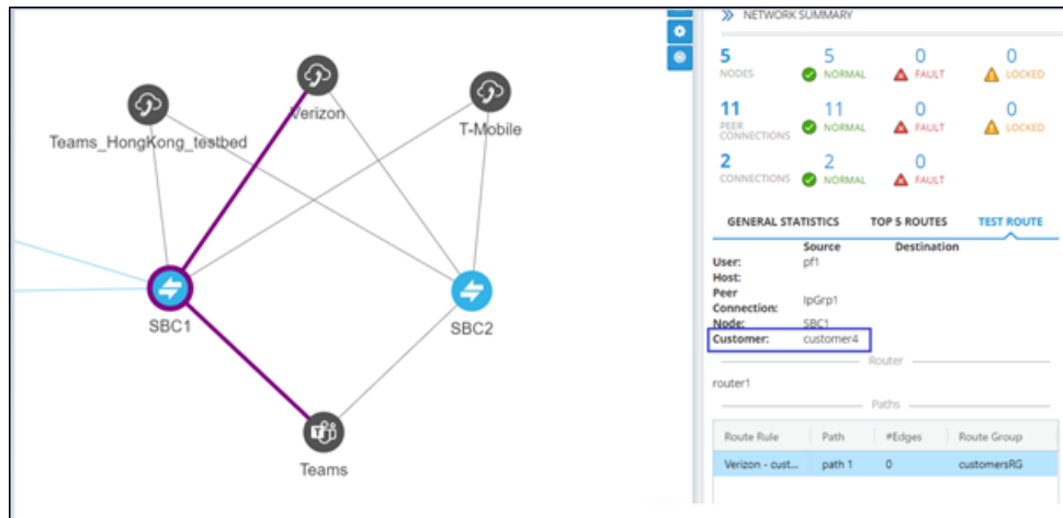
Figure 3-39: Testing a Route from a 'Customer' Entity
