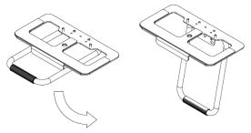
3. Place the RXV81 and the bracket on top of the TV screen and clamp the bracket to the TV screen.
