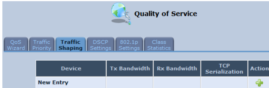
Figure 11-2: Quality of Service – Traffic Shaping Screen
