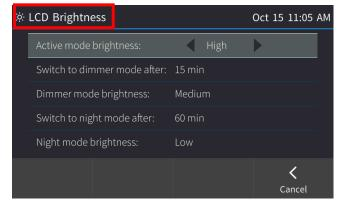
Users can configure a brightness level of High, Medium or Low for Active mode, Dimmer mode and Night mode. By default, the phone enters Dimmer mode after 15 minutes of inactivity; by default, the phone enters Night mode after another 60 minutes of inactivity. If the capability to determine working hours is configured, the phone only enters Night mode during non-working hours.
