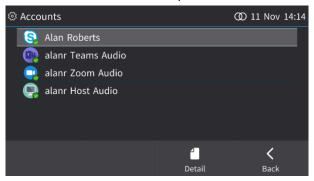
A new Accounts screen shown in the preceding figure allows users to view the status of their accounts and paired applications. The screens of the 450HD and 445HD are like the C450HD screen shown here, with insignificant differences.
