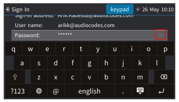
By default, the password is *masked*, and the icon is an *open* eye indicating that if the user clicks it, the password will be *unmasked* for the user to make sure their input was correct. When the password is *unmasked*, the eye icon is *struck through*.
