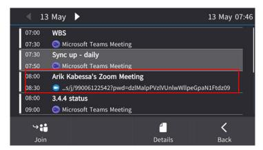
Users can **join a Zoom meeting** by selecting it in the phone Calendar (identified by the Zoom icon) and then selecting the **Join** softkey, as shown in the next figure. The 'Join' is performed as 'automatic dial-in'.
