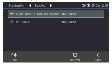
Press the Pair softkey to pair the device. After pairing is complete, the phone displays 'Connected'.
