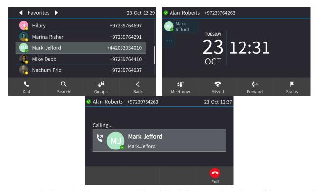
The figures show the Favorites screen [upper left] including a contact's initials instead of their picture, the idle screen [upper right] with a speed dial to a contact, and the Calling screen [lowermost].
