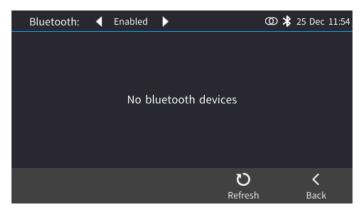
• Configure the device (Bluetooth headset or speaker) to allow pairing and then press the **Refresh** softkey; the phone attempts to discover available devices:
