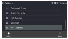
• Wi-Fi is disabled by default. Wi-Fi is enabled | disabled by pressing the right rim | left rim of the navigation button on the phone:
