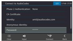
After configuring the Wi-Fi parameters, the user presses the Connect softkey again and waits about 20-30 seconds for the phone to connect to Wi-Fi and receive an IP address; the Wi-Fi icon is then displayed in the uppermost right corner of the screen:
