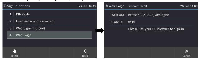
The parameter 'Secure (HTTPS) communication' in AudioCodes' IP Phone Manager Pro/Express management interface must be enabled for the Web Login feature to function.
